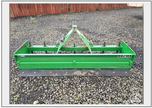
**Description** Has 2 blades, 1 for pushing and 1 for pulling. 3 point attachment, Model number BB2184.
